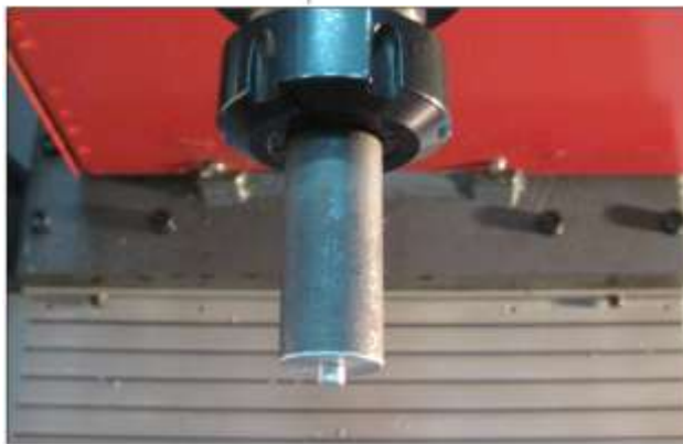
Fig.6 Straight type pin tool attached with FSW machine
